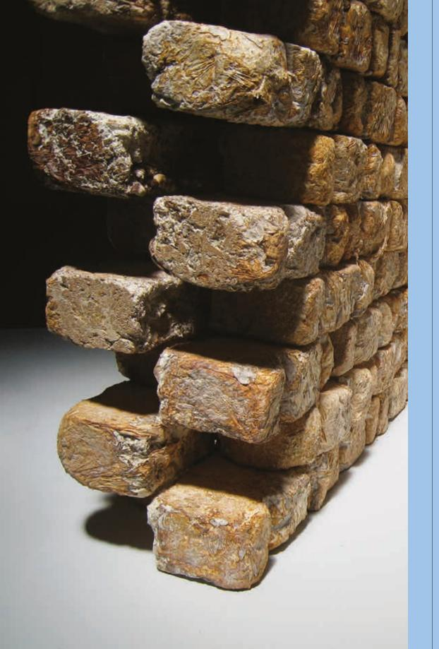
Mycotecture bricks are bricks that are grown out of a living fungus. The fungus digests and binds together smaller pieces of organic materials into a tightly bound structure. Though incredibly strong and durable, fungal materials can readily be broken down with a range of benign processes and incorporated back into the world.
