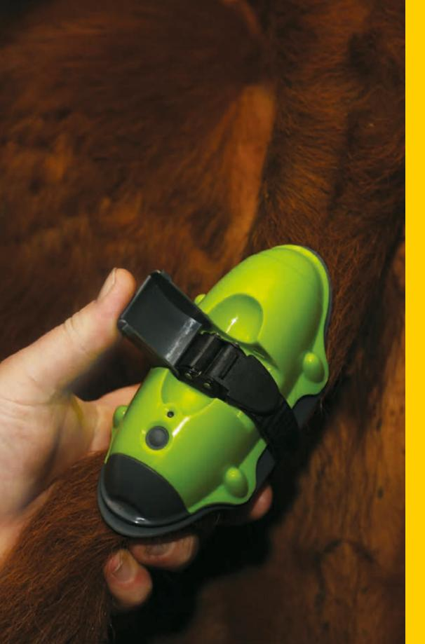
*Moocall* is a calving sensor worn on a cow's tail that measures over six hundred data points every second to determine the onset of calving. The device then sends a text alert to two mobile phones roughly an hour before calving, to ensure that the cattle breeder can be on location when a calf is born.
