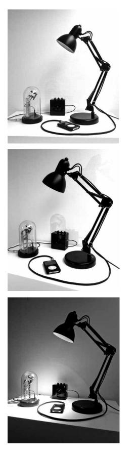
This project was inspired by Alexander Graham Bell's wireless communication research which allowed him to transmit and receive sound through a modulated beam of light. *AM Audio Desk Light* is a personal version of Bell's research applied to a regular black desk lamp. The audio output of an MP3 player is wirelessly transmitted to a photocell (an electronic device that generates electricity when light falls on it) via a flickering LED light.
